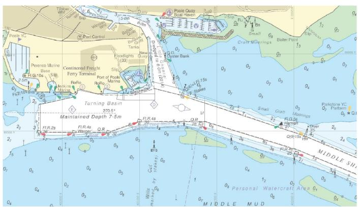
The areas to be dredged are the 'Turning Basin' and the 'Little Channel' and all spoil will be deposited at the Swanage spoil ground.
