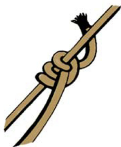
Taut-Line or Rolling Hitch
